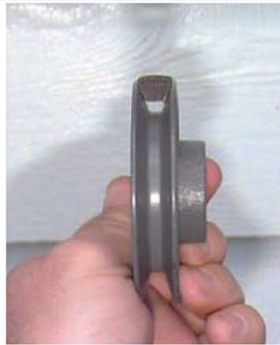
Figure 2. A new fan belt rides high in the pulley so that the top of the belt rides just above the top of the pulley.
